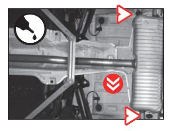
Remove the rubber brackets and unscrew the actuator of the rear exhaust.
